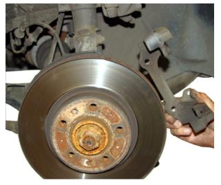
Remove the carrier and inspect for damage and corrosion.
