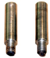
Using TRW Brake Cleaner, clean and examine the guide pins. Dirty, corroded or worn guide pins will affect the sliding ability of the caliper housing. A seized or partially seized Caliper can result in poor braking efficiency, overheating or disc damage.
