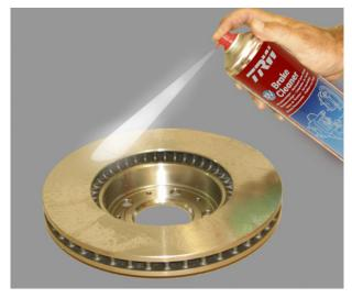
Degrease all surfaces of the new disc. Take care when handling the clean disc and ensure no grease/dirt is transferred to the clean surfaces.
