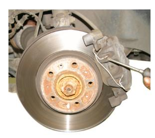
Release the spring from the second location point and remove from the caliper.
