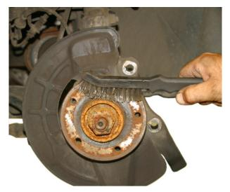
Clean the wheel hub with a wire brush. TRW Brake Cleaner will help to prevent brake dust. Always wear safety glasses to prevent injury.
