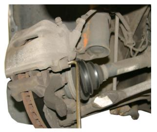
Remove both guide pins. Typically a 7 mm hexagon Allan key will be required.
