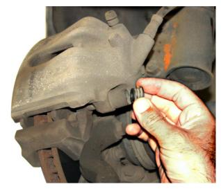
Remove both guide pin dust caps and check their condition. It is vital for the correct function of this brake system that the dust cap is not damaged. Water and dust ingress will lead to corrosion, which will affect the brake sliding ability. This can result in poor braking efficiency, overheating or disc damage.
