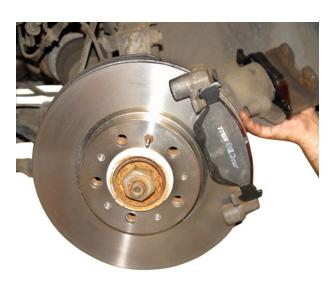
Fit the new outer/inner brake pads into the carrier. For some applications the positioning of the pads is dependent on the direction of disc rotation. If in doubt refer to the Vehicle Manufacturers recommendation.
