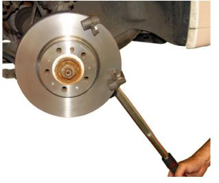
Refit the carrier and ensure the retaining bolts are tightened to the torque level specified by the Vehicle Manufacturer.
