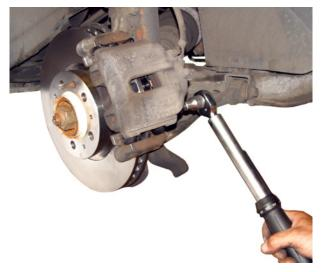
Locate the housing correctly on the carrier, ensure the pads remain correctly located. Fit the guide pins and tighten to the torque level specified by the Vehicle Manufacturer.
