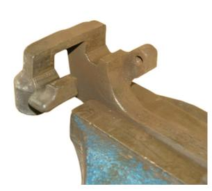
Clean the carrier following the procedure detailed for the wheel hub. Pay particular attention to the pad abutment faces.
