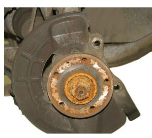
Examine the disc mounting face on the hub for corrosion or damage, including the threads.
