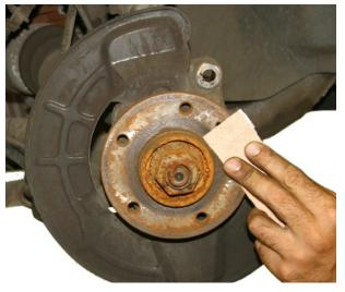
In some cases it may be necessary to use abrasive paper to remove corrosion from the hub. Take care not to remove metal from the hub face. Never use grinding tools. They will destroy the surface of the hub
