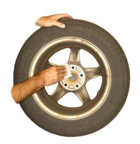
Clean the hub contact surface of the road wheel. Clean the wheel inside and outside, this will help prevent vibrations due to imbalance. Avoid heavy braking for the first 200Km, 125 mikes
