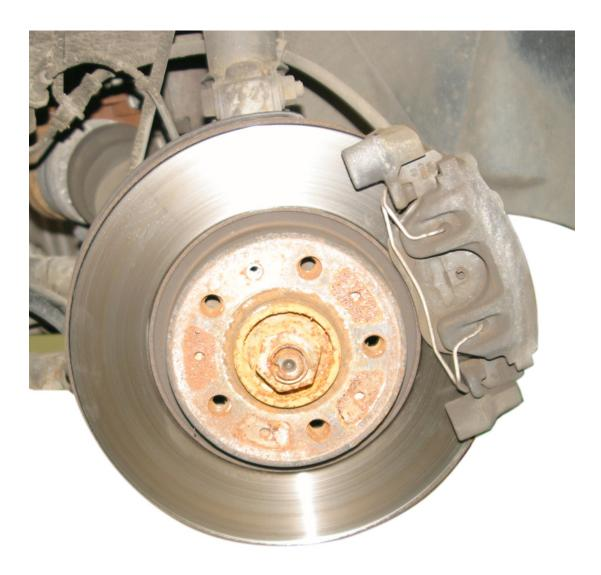
A generic example how to change discs and pads on a front application incorporating the TEVES FN-type Caliper
