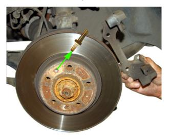
Where applicable, remove the disc retaining screw. Remove the disc.
