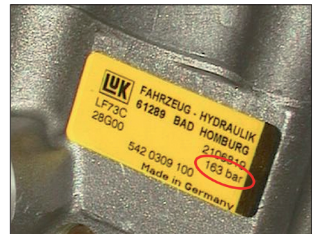
LuK power-steering pump with pressure control valve
