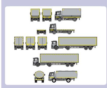
This is a large and complicated change that we have made. It introduces **Conspicuity**Marking into the test and appropriate marking on the rear and sides of the vehicle are required.
