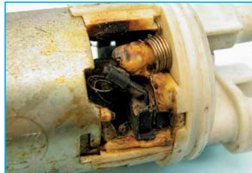
Damage as a result of running dry
